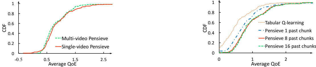
Figure 13: Comparing ABR algorithms trained across multiple videos with those trained explicitly on the test video. The measuring metric is QoE_{lin} .
